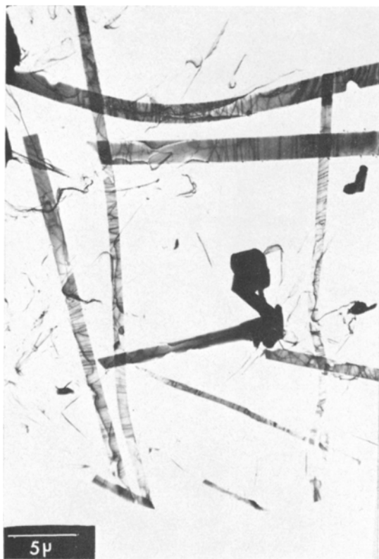
Figure 22 Coherent whiskers (TFI) after 4 h at 1400°C.
