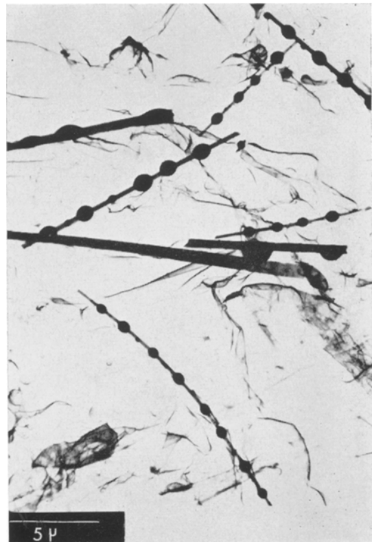
Figure 15 Spheroidisation (CTH whiskers) after 17 h at 1100°C.
