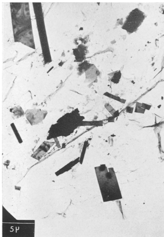
Figure 16 CTH whisker fragmentation after 4 h at 1300°C.
