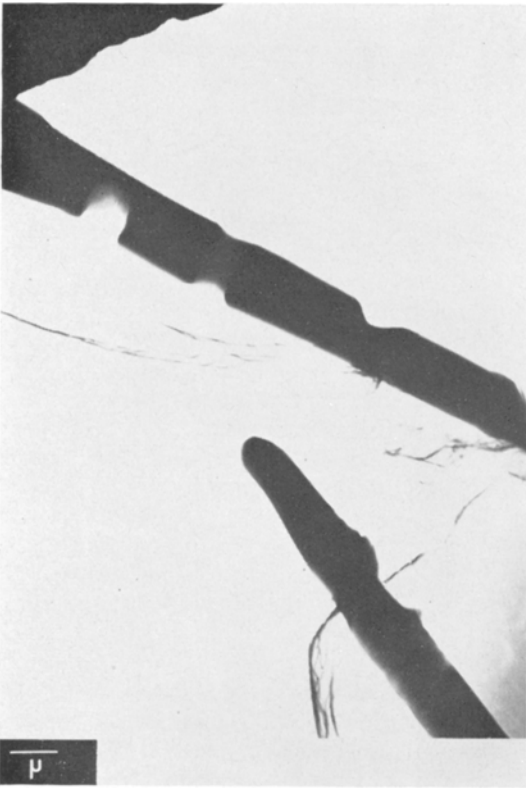
Figure 18 Surface pits (CTH whiskers) after 4 h at 1500°C.
